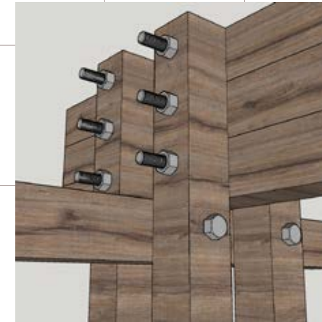
CONNECTION OF COLUMNS WITH BEAMS
