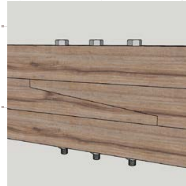
SCARF JOINT CONNECTION
