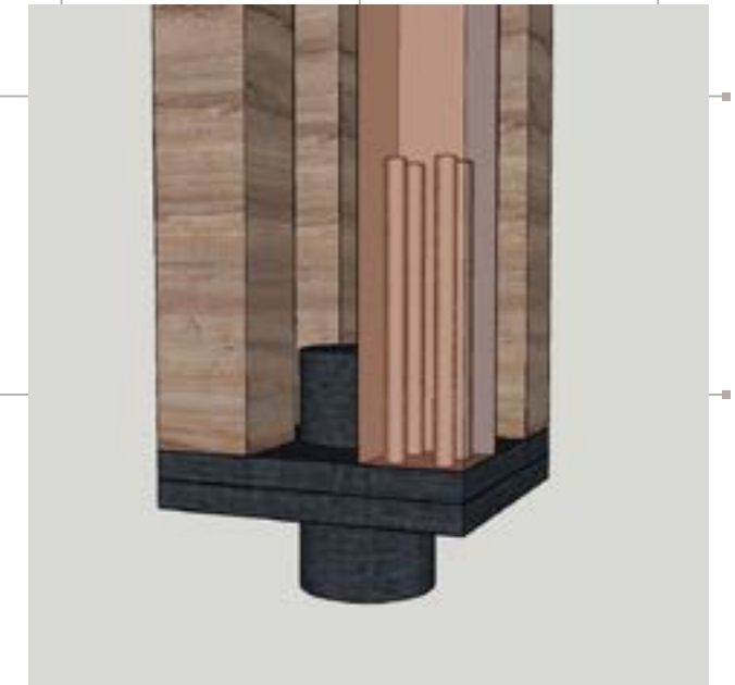
CONNECTION OF BASE PLATE WITH TIMBER COLUMNS
