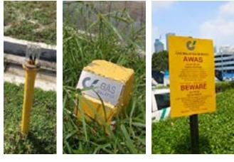
STONE MARKERS, TEST POST AND WARNING SIGNS BY GAS MALAYSIA BERHAD INDICATES THERE'S AN EXISTING GAS PIPELINE UNDERGROUND. TEST POST ARE FOR TESTING THE **CORROSSION LEVEL** OF THE GAS PIPES (MIDF, 2016)
